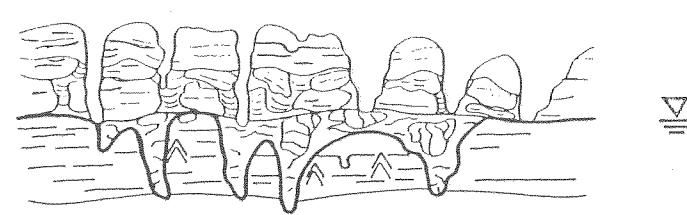
T-10 ENLARGED PITS AND PIPES AND HUMMOCKY RELIEF DEVELOPS FOLLOWING A LARGE WATERTABLE DROP.
